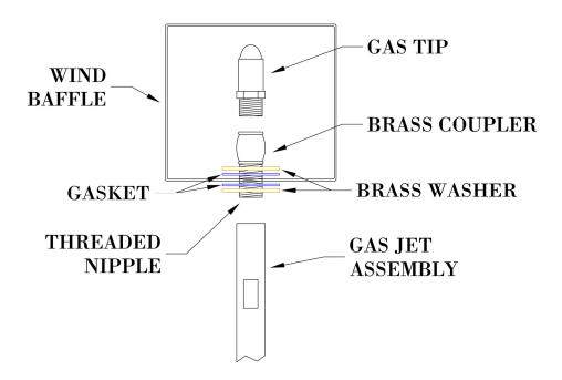
Step 4: Return gas valve to open position and relight burner. Bevolo recommends flame height to be 1" -1 ½" for smaller fixtures.
